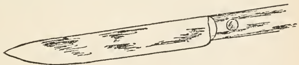
CONVEX OR ROCKER-SHAPED CUTTING EDGE
